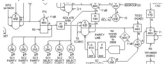
Most of the symbols represent neurons. Each neuron symbol has a number and a Greek letter which, together with the box label, creates a unique identifier. Neurons with a  $1\mu$ s delay, called "half neurons", are represented by circular symbols. Neurons with a  $2\mu$ s delay, "full neurons", are represented by square symbols. (Remember, it's the external timing signals which determine the delay. There is no physical difference in the neurons.)
