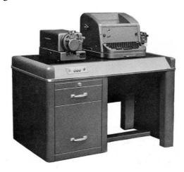
Programmers prepared programs and data by writing them on paper. Then they sat at a teleprinter desk like this one to type them in, thus getting a printed hard copy and a simultaneously-punched paper tape for input to the Sirius computer. The printed version would be checked for typing errors.
