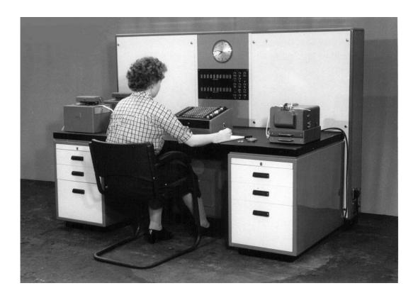
In this photograph the clock and display panel can be seen set into the mainframe cabinet.
